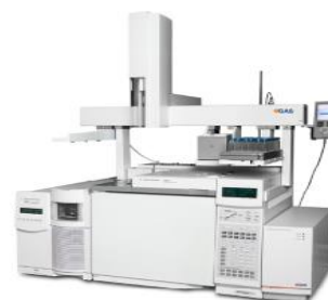
Fig. 2. Agilent 6890N GC with 5973 MSD (Agilent) and IMS (G.A.S.)
