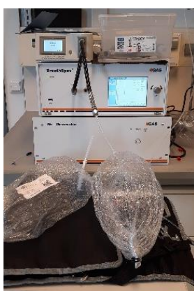
Fig. 3. Coupling of \mu -TD (AIRSENSE) with GC-IMS plus N 2 -Generator (G.A.S.)
