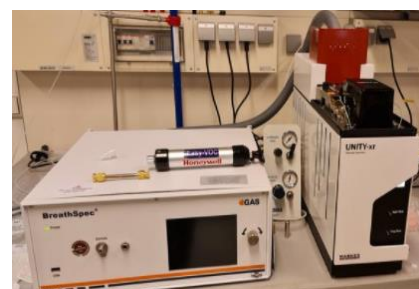
Fig. 4. BreathSpec® (G.A.S.) coupled to a Thermal Desorber (MARKES Unity-xr).
